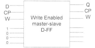
Fig. 4.2.3: Block diagram of Reversible Write-Enabled Master-Slave D-FF
