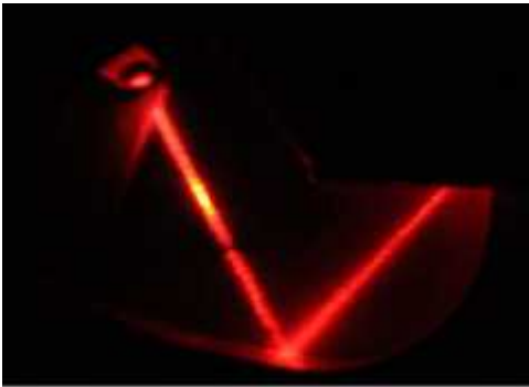
Fig. 9: (c) Test-2 Laser ray on circular reflector of CTAH
