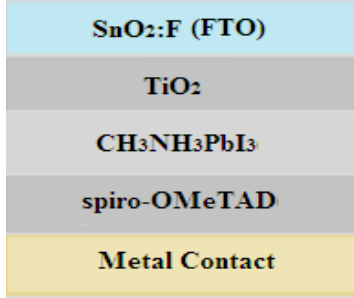
Fig. 1: Model of Perovskite Solar Cell. ( \text{TiO}_2 as ETM, Perovskite ( \text{MAPbI}_3 ) as absorber and spiro-OMeTAD as HTM).
