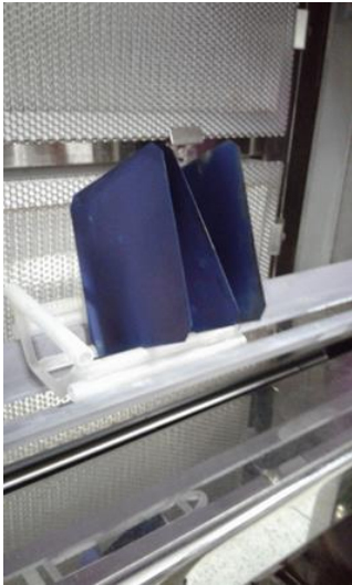
Fig. 4: Phosphorus Doped Wafer Unloaded From Furnace
