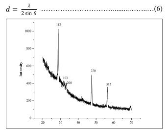
**Fig. 4.** The XRD patterns of the sulfurized CZTS thin films prepared from the chloride chemical based precursor.
