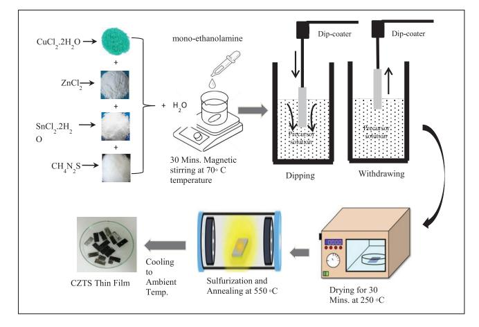
Fig. 1. Synthesis process of CZTS thin films is laid-out in the diagram: preparation of precursor solution, deposition of CZTS films on glass substrate through dip coating method, drying and annealing. The deposited CZTS thin films are finally presented in a petri dish in the diagram.
