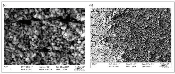
Fig. 5. The surface morphology of the CZTS thin film [(a) 25000X (b) 500X].
